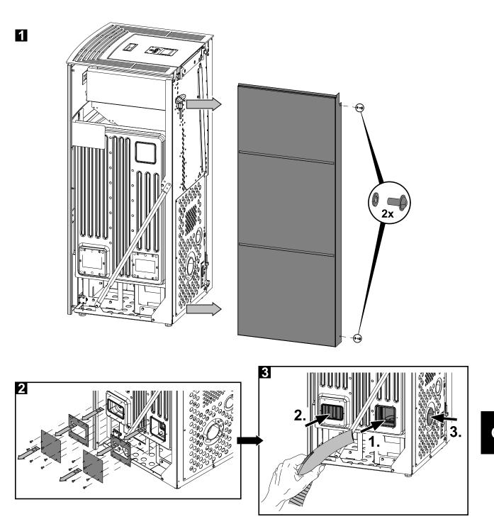
Figure 3a: Removing the side wall (HSP 6 Rueda PGI)
