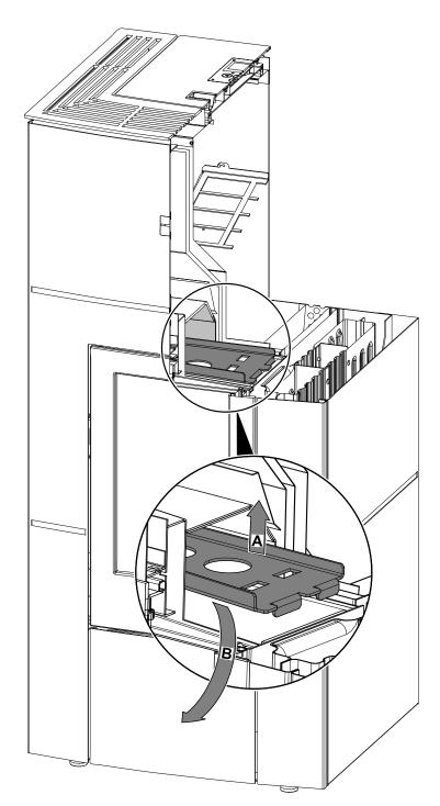
Figure2: Removing the flue baffle
