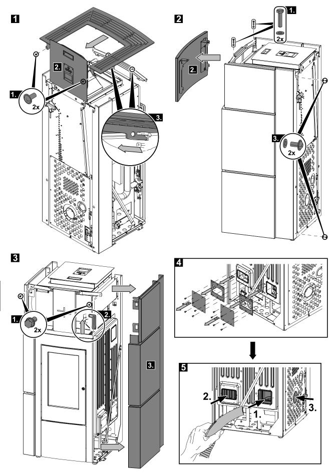
Figure 3c: Removing the side wall (HSP 6 Rueda C PGI)
