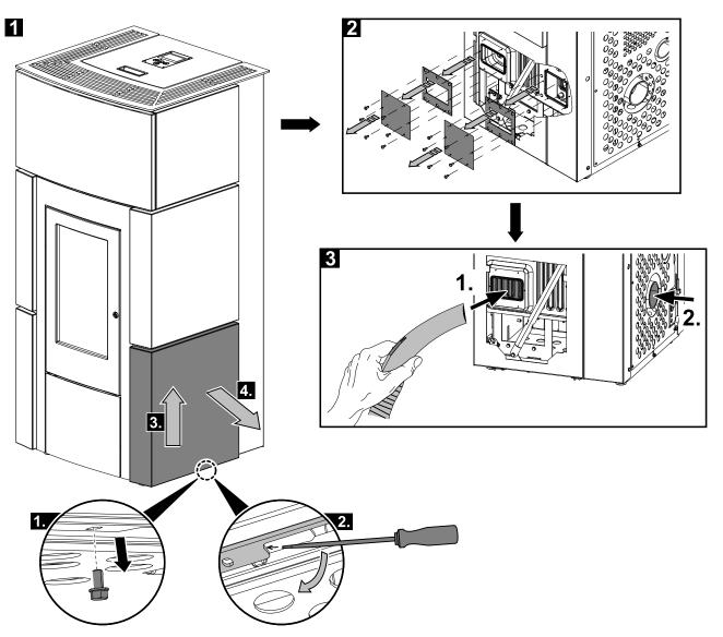
Figure 3b: Removing the side wall (HSP 6 Rueda C PGI)
