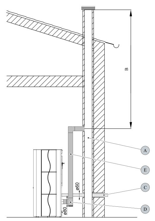
Figure 1.3: Connection to the existing chimney
